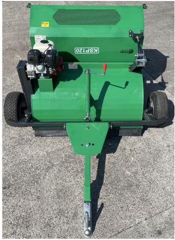
Engine-powered sweeper for leaves, grass and rubbish. For ATVs or compact tractors with 50 mm tow bar ball hitch. Stiff brushes effectively sweep up loose materials and discharge them into the collector that holds approx. 500 l/150 kg.
